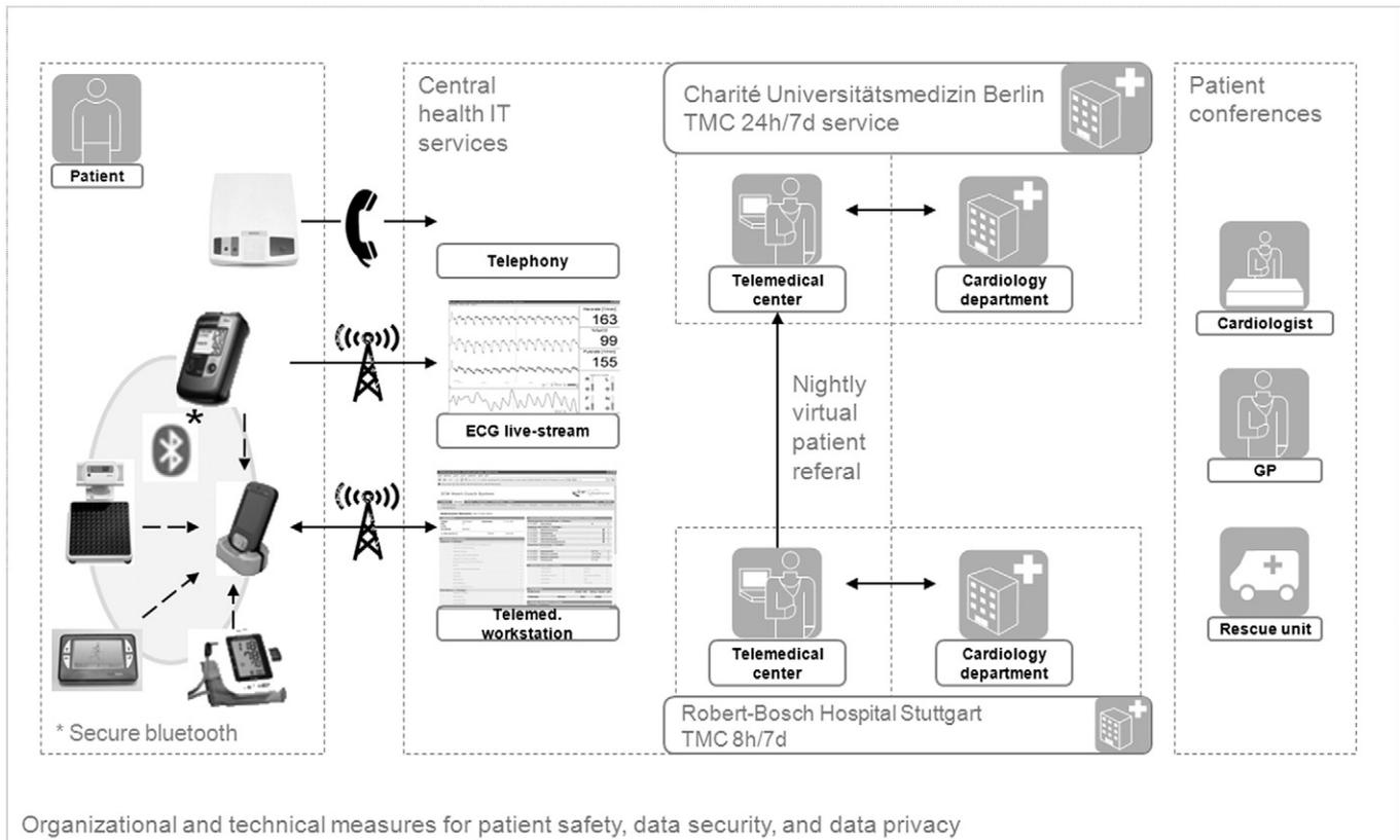
**Fig. 1.** Telemonitoring system and structure of service. Devices for ECG, blood pressure and weight are connected via Bluetooth® at the patient's home. A PDA transmits the data via its integrated mobile phone module to the central servers. There are two telemedical centres in hospitals for disease management communicating through an electronic patient record. A home emergency call system enables direct patient contact with the specialist.
