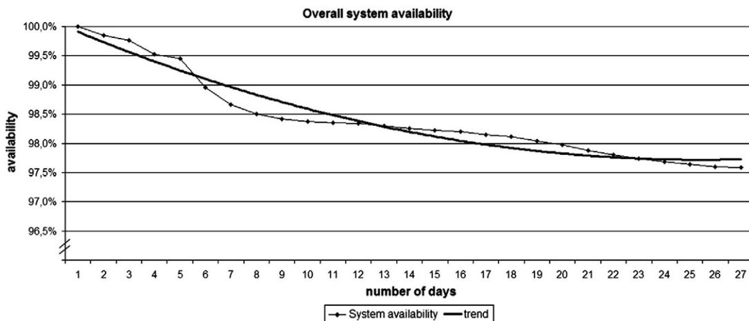
**Fig. 3.** Total system availability, measured as up-time of all central hardware components including mobile phone network and key software elements.
