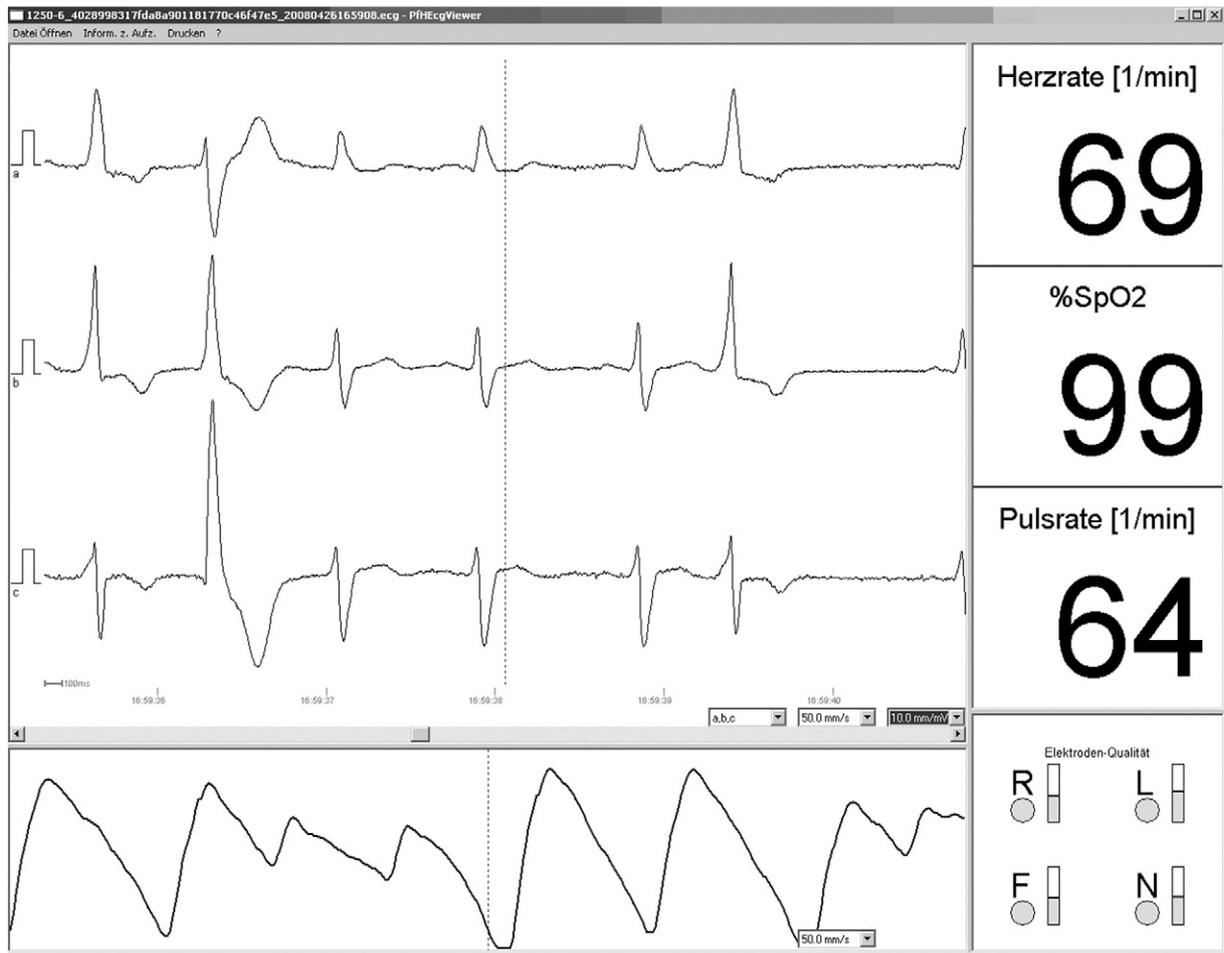
**Fig. 2.** Detail of continuous ECG monitoring (live stream). ECG and plethysmograph waveforms as well as values for heart rate, arterial oxygen saturation (%SpO2) and information about electrode contact are shown in a web-based viewer.
